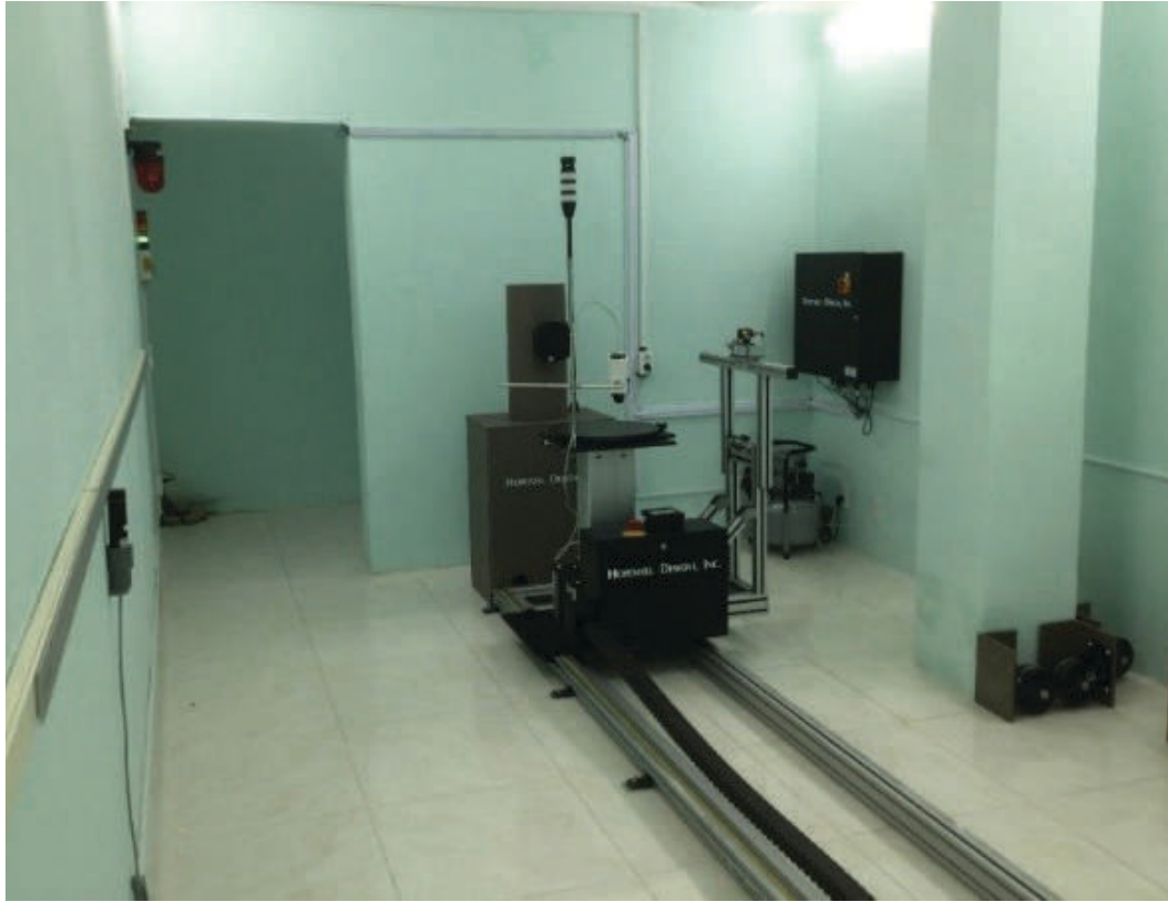
Standard dosimetry laboratory using Cesium-137 Gamma Source
