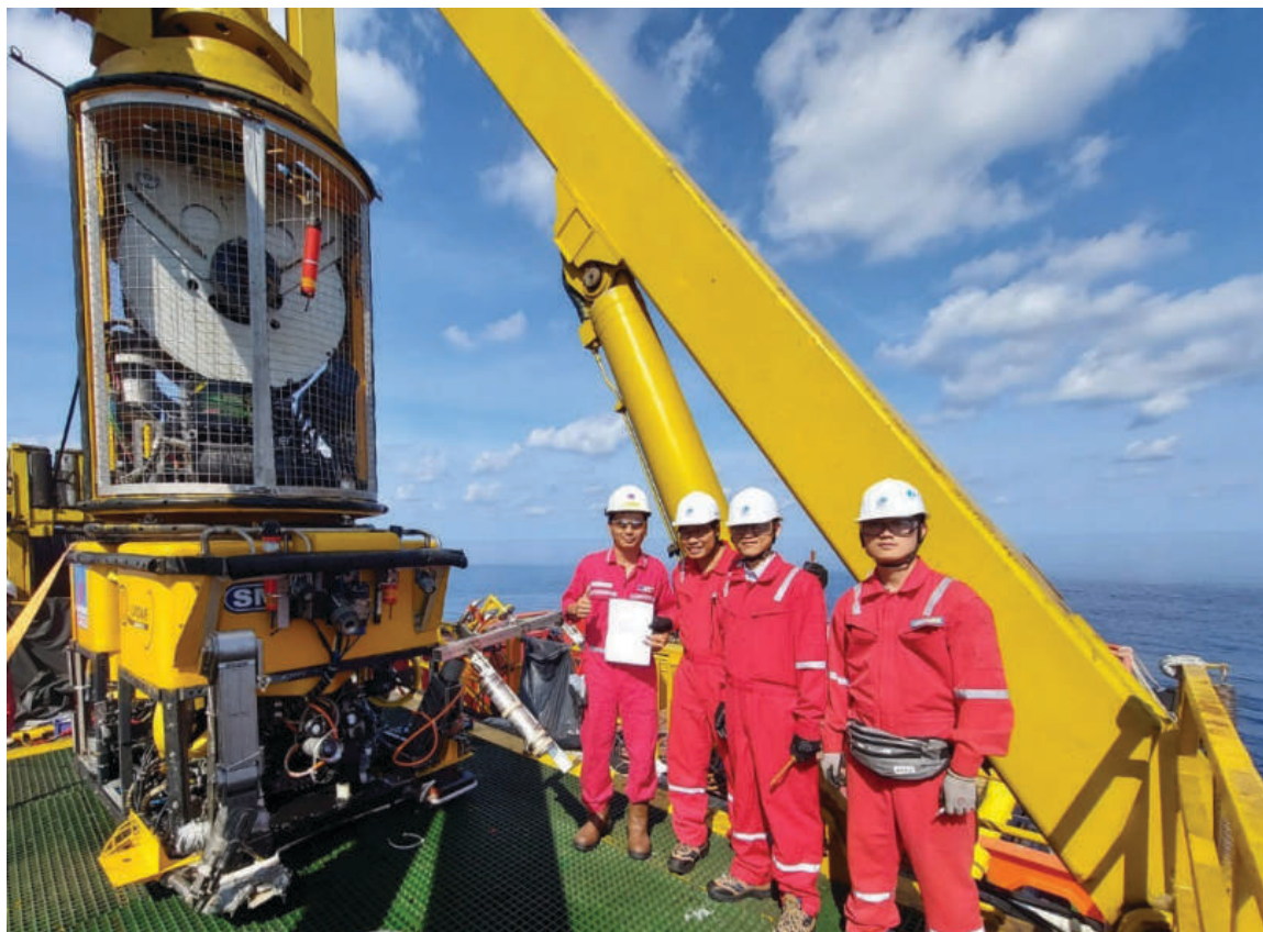
Deployment of Flooded member detection (FMD) inspection service at Chim Sao mine
