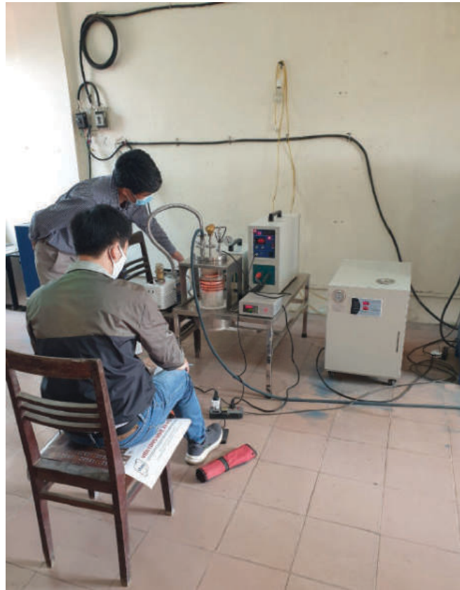
Using vacuum induction furnace to prepare rare earth metals
