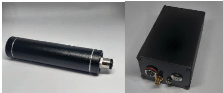
Figure 1. NaI(Tl)+SiPM detector and single-channel measuring system for this type of probe
