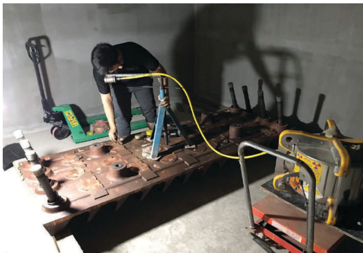
Quality inspection and evaluation of large-thickness castings for special materials by high-energy gamma source (Co-60)
