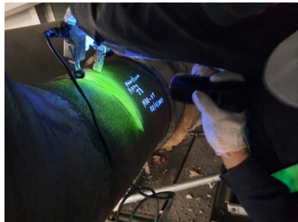
Figure 3. Fluorescence wet magnetic particle testing
