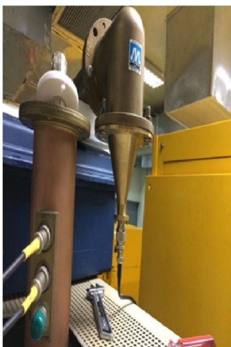
Connect the waveguide and adjust the RF system for the KOTRON-13 Accelerator device within the framework of a ministerial-level project
