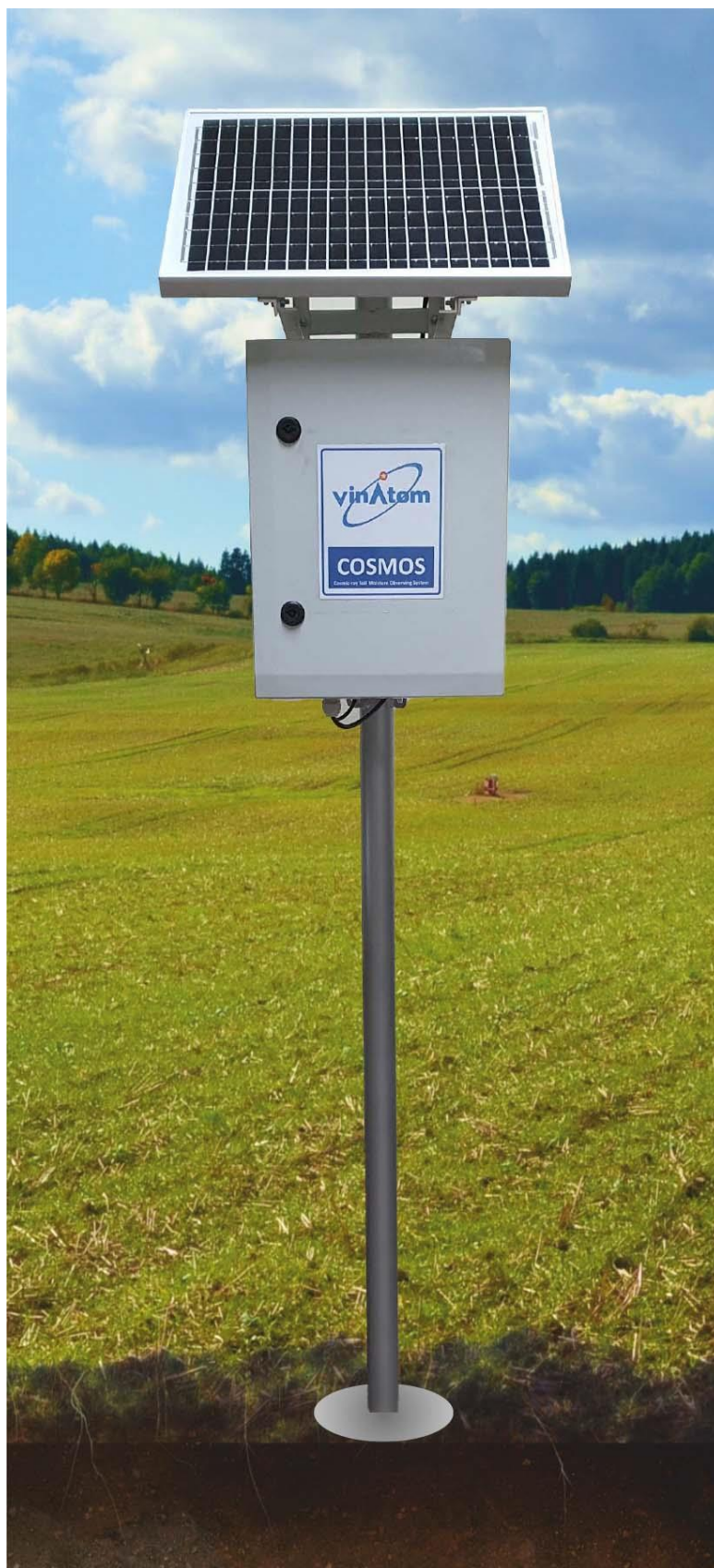
COSMOS-VINATOM System-Cosmic-ray Soil Moisture Observing System (Ministerial Project of 2021-2022)
