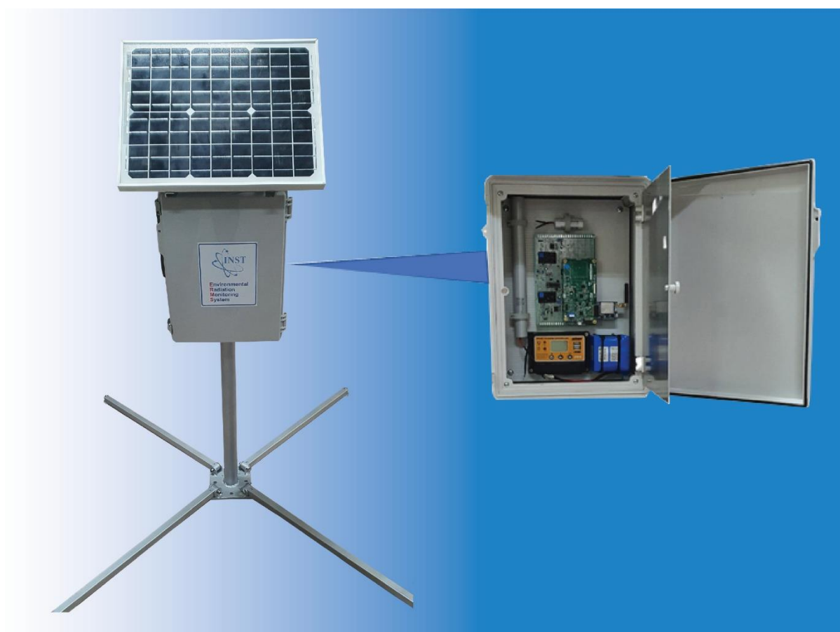
Environmental radiation monitoring system VinaERMS-INST have installed in Lang Son
