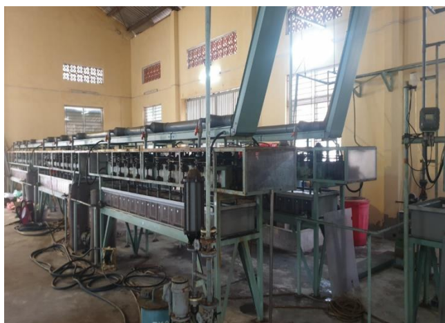
(a) Box-type mixer-settler 120 stage-system (Japan supported)
