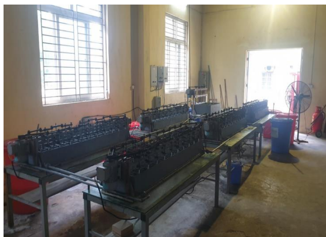
(b) Box-type mixer-settler 100 stage-system (Vietnam manufactured)
