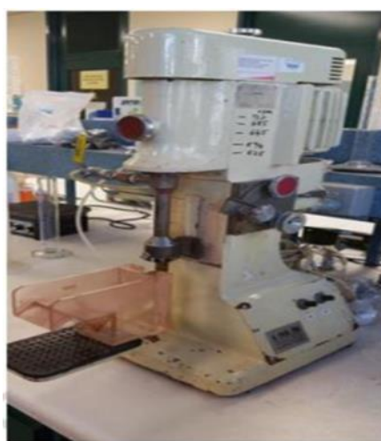
Figure 3. Denver flotation machine for mineral flotation tests
