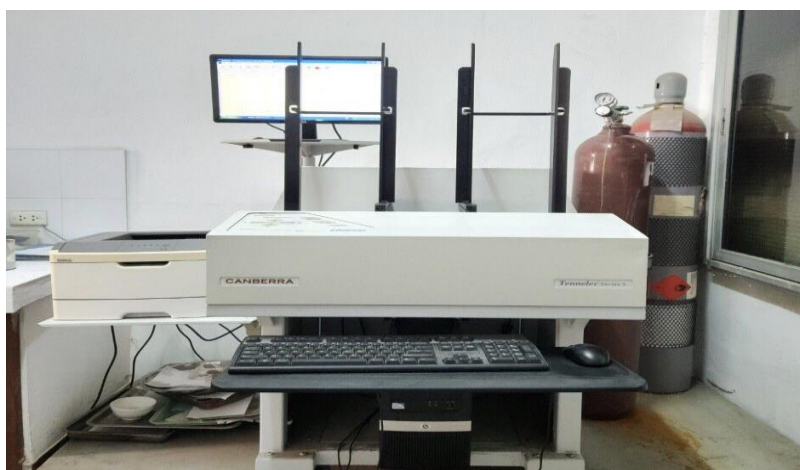
Figure 1. LB5500 alpha and beta total radioactive activity measuring device
