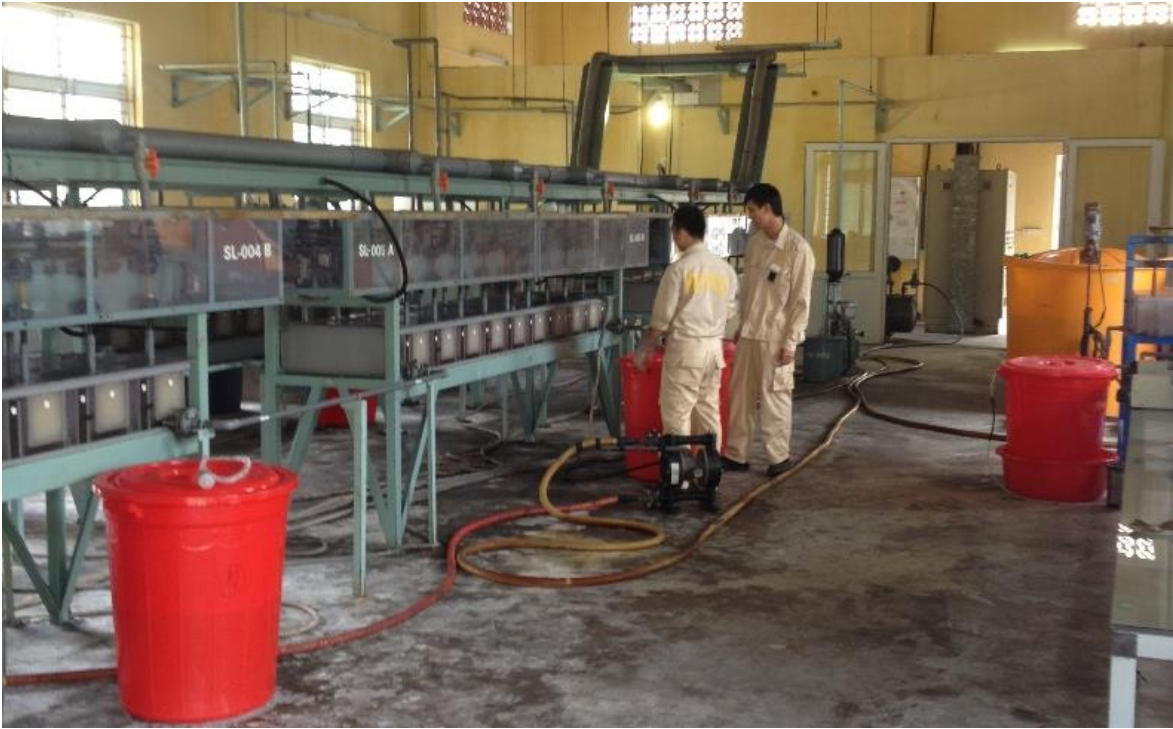
Operating separately RE extraction systems at Phung campus
