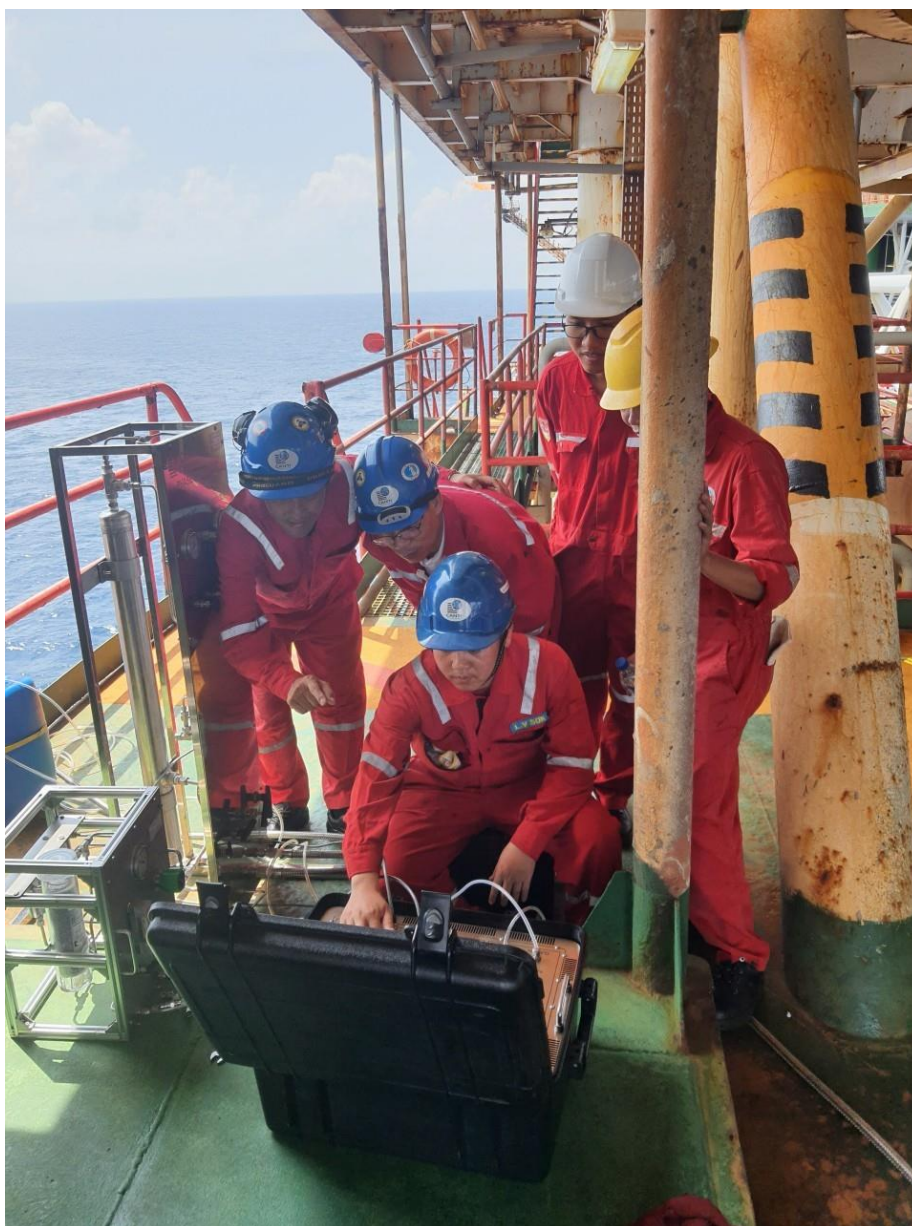
Application of the leak control method for gas-lift wells using the chemical tracer technique in the Bach Ho oil field.
