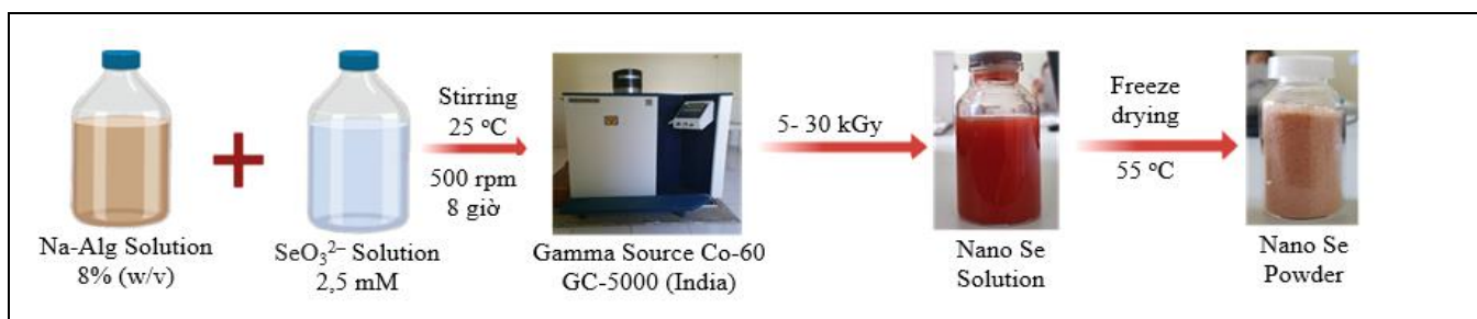
Figure 1. Process of nano selenium synthesis by gamma irradiation technology
