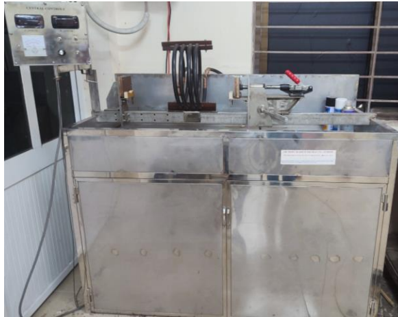
Figure 1. The stationary magnetic particle testing system
