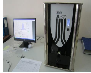
Figure 3. The TLD reader system - REXON UL-320
