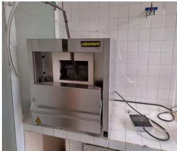
Figure 1. Nabertherm N7/H furnace
