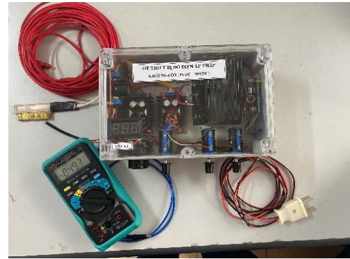
Figure 1. DC power supply and low voltage test probe
