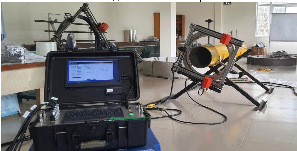
Clamp- on first-generation CT scanner (gORBIT-140)
