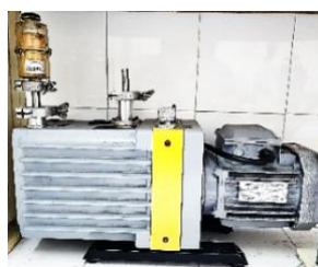
Figure 7. Two-Stage Vacuum Pump HBS 2XZ – 6
