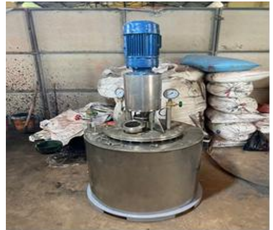
Figure 2. 20kg/batch pressure apparatus
