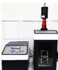
Figure 6. High-Power Ultrasound Device FS-1800N
